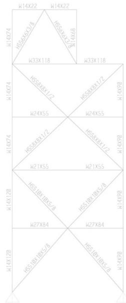
Figure 15 BF-NS-2 Frame Sections
